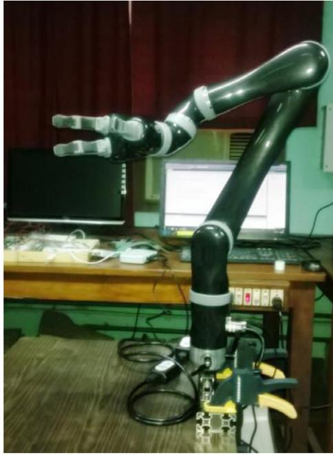
Fig. 2. Jaco Robot Arm setup in our lab.
